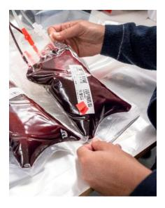
Picture: One of the new PVC-free blood bags filled with blood and ready for further tests.
